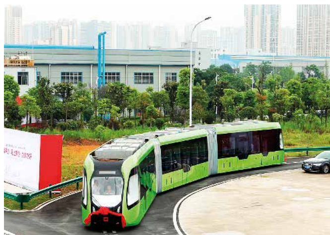
Figure 23: CRRC’s optically-guided bus (trackless tram) now operating in Zhuzhou (Hebei, China)
