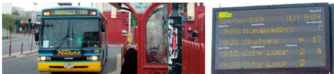
Figure 7: Distinctive SmartBus vehicles and real-time stop infrastructure
