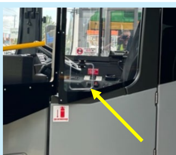
Figure 13: Example of access hole or portal hole.
