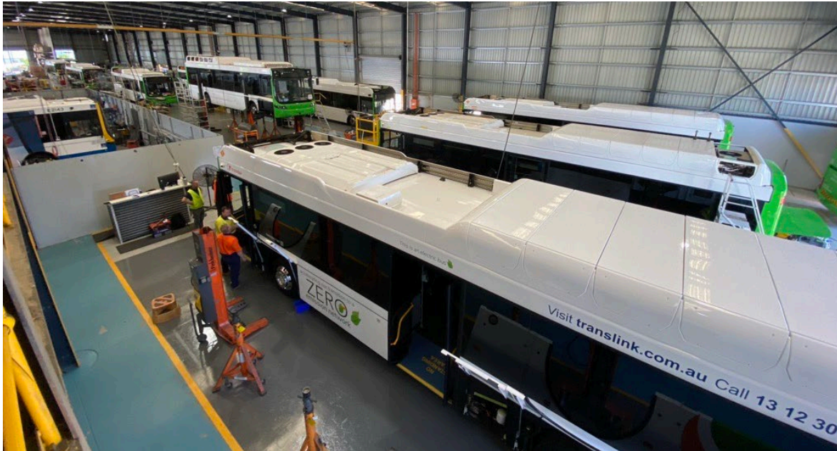
Zero emission buses in construction at a Factory in Brisbane
